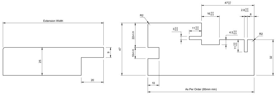
Extension Head length = Lining Head Length Extension Head Rebate length = Extension Head -50mm Extension Head Rebate depth = 9mm Extension Jamb length = Lining Jamb Length +15mm
